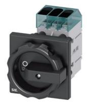
Load disconnector 3LD3, lu 25 A Main switch 3-pole Rated operating capacity at AC-23 A at 400V 9.0kW Front plate mounting Basic switch with Central hole mounting 22.5mm Toggle drive black 66x66 mm
