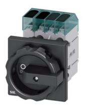
Load disconnector 3LD3, lu 25 A Main switch 3-pole + N Rated operating capacity at AC-23 A at 400V 9.0kW Front plate mounting Basic switch with Central hole mounting 22.5mm Toggle drive black 66x66 mm
