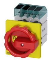
Load disconnector 3LD3, lu 25 A Main switch 3-pole + N Rated operating capacity at AC-23 A at 400V 9.0kW Front plate mounting Basic switch with Central hole mounting 22.5mm Toggle drive red / yellow 66x66 mm
