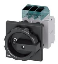
Load disconnector 3LD3, lu 25 A Main switch 3-pole Rated operating capacity at AC-23 A at 400V 9.0kW Front plate mounting Basic switch with Central hole mounting 22.5mm Toggle drive black 66x66 mm with auxiliary switch 1OE + 1S
