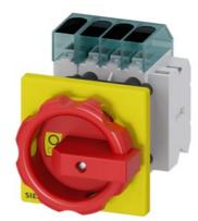
Load disconnector 3LD3, lu 25 A Main switch 3-pole + N Rated operating capacity at AC-23 A at 400V 9.0kW Front plate mounting Basic switch with Central hole mounting 22.5mm Toggle drive red / yellow 66x66 mm with auxiliary switch 10E + 1S
