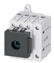
Load disconnector 3LD3, lu 32 A Main switch 3-pole + N Rated operating capacity for AC-23 A at 400V 11.5kW Installation in distribution boards, Basic switch without Knob-operated mechanism
