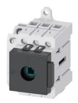
Load disconnector 3LD3, lu 32 A Main switch 3-pole Rated operating capacity for AC-23 A at 400V 11.5kW Installation in distribution boards, Basic switch without Knob-operated mechanism with auxiliary switch 1OE + 1S
