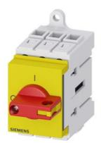
Load disconnector 3LD3, lu 32 A Main switch 3-pole Rated operating capacity for AC-23 A at 400V 11.5kW Installation in distribution boards, Basic switch with selector knob red / yellow
