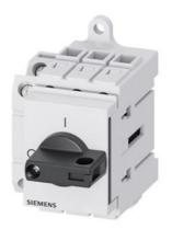
Load disconnector 3LD3, lu 32 A Main switch 3-pole Rated operating capacity for AC-23 A at 400V 11.5kW Installation in distribution boards, Basic switch with selector knob black with auxiliary switch 1OE + 1S
