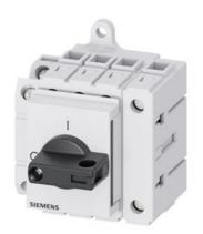
Load disconnector 3LD3, lu 32 A Main switch 3-pole + N Rated operating capacity for AC-23 A at 400V 11.5kW Installation in distribution boards, Basic switch with selector knob black with auxiliary switch 1OE + 1S
