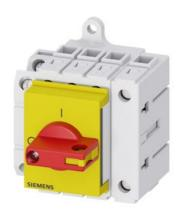
Load disconnector 3LD3, lu 32 A Main switch 3-pole + N Rated operating capacity for AC-23 A at 400V 11.5kW Installation in distribution boards, Basic switch with selector knob red / yellow with auxiliary switch 1OE + 1S
