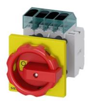
Load disconnector 3LD3, lu 16 A Main switch 3-pole + N Rated operating capacity at AC-23 A at 400V 7.5kW Front plate mounting Basic switch with Central hole mounting 22.5mm Rotary actuator red / yellow 66 x 66 mm with auxiliary switch 1OE + 1S
