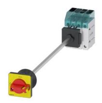
Load disconnector 3LD3, lu 32 A Main switch 3-pole + N Rated operating capacity for AC-23 A at 400V 11.5kW floor mounting Basic switch with door coupling Central hole mounting 22.5mm Toggle drive red / yellow 48x48 mm
