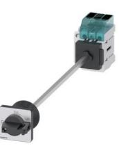
Load disconnector 3LD3, lu 32 A Main switch 3-pole Rated operating capacity for AC-23 A at 400V 11.5kW floor mounting Basic switch with door coupling Central hole mounting 22.5mm Toggle drive black 48x48 mm with auxiliary switch 10E + 1S
