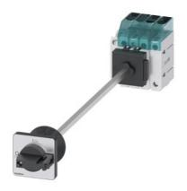
Load disconnector 3LD3, lu 32 A Main switch 3-pole + N Rated operating capacity for AC-23 A at 400V 11.5kW floor mounting Basic switch with door coupling Central hole mounting 22.5mm Toggle drive black 48x48 mm with auxiliary switch 10E + 1S
