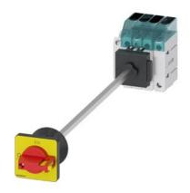
Load disconnector 3LD3, lu 32 A Main switch 3-pole + N Rated operating capacity for AC-23 A at 400V 11.5kW floor mounting Basic switch with door coupling Central hole mounting 22.5mm Toggle drive red / yellow 48x48 mm with auxiliary switch 10E + 1S
