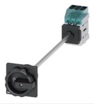
Load disconnector 3LD3, lu 32 A Main switch 3-pole Rated operating capacity for AC-23 A at 400V 11.5kW floor mounting Basic switch with door coupling Central hole mounting 22.5mm Rotating drive black 66 x 66 mm
