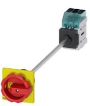
Load disconnector 3LD3, lu 32 A Main switch 3-pole Rated operating capacity for AC-23 A at 400V 11.5kW floor mounting Basic switch with door coupling Central hole mounting 22.5mm Rotary actuator red / yellow 66 x 66 mm
