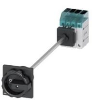
Load disconnector 3LD3, lu 32 A Main switch 3-pole + N Rated operating capacity for AC-23 A at 400V 11.5kW floor mounting Basic switch with door coupling Central hole mounting 22.5mm Rotating drive black 66 x 66 mm
