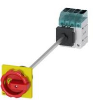
Load disconnector 3LD3, lu 32 A Main switch 3-pole + N Rated operating capacity for AC-23 A at 400V 11.5kW floor mounting Basic switch with door coupling Central hole mounting 22.5mm Rotary actuator red / yellow 66 x 66 mm
