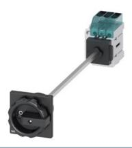
Load disconnector 3LD3, lu 32 A Main switch 3-pole Rated operating capacity for AC-23 A at 400V 11.5kW floor mounting Basic switch with door coupling Central hole mounting 22.5mm Rotating drive black 66 x 66 mm with auxiliary switch 1OE + 1S
