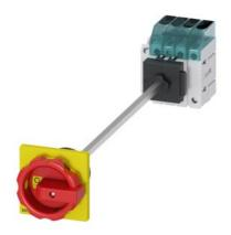
Load disconnector 3LD3, lu 32 A Main switch 3-pole + N Rated operating capacity for AC-23 A at 400V 11.5kW floor mounting Basic switch with door coupling Central hole mounting 22.5mm Rotary actuator red / yellow 66 x 66 mm with auxiliary switch 10E + 1S
