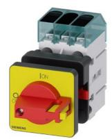
Load disconnector 3LD3, lu 32 A Main switch 3-pole Rated operating capacity for AC-23 A at 400V 11.5kW Front plate mounting Basic switch with Central hole mounting 22.5mm Toggle drive red / yellow 48x48 mm
