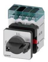
Load disconnector 3LD3, lu 32 A Main switch 3-pole + N Rated operating capacity for AC-23 A at 400V 11.5kW Front plate mounting Basic switch with Central hole mounting 22.5mm Toggle drive black 48x48 mm
