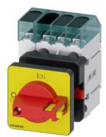
Load disconnector 3LD3, lu 32 A Main switch 3-pole + N Rated operating capacity for AC-23 A at 400V 11.5kW Front plate mounting Basic switch with Central hole mounting 22.5mm Toggle drive red / yellow 48x48 mm
