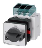
Load disconnector 3LD3, lu 32 A Main switch 3-pole Rated operating capacity for AC-23 A at 400V 11.5kW Front plate mounting Basic switch with Central hole mounting 22.5mm Toggle drive black 48x48 mm with auxiliary switch 10E + 1S
