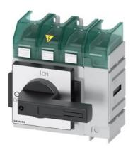
SENTRON, Molded case switch 3LD5 UL, Main switch, 4-pole, certified according to UL489 UL60947-4-1 and IEC60947-3, UL: 100A, SCCR 65kA at 480VAC, Operating power at 480VAC 3-phase: 60hp, IEC: 100A, Operating power at AC-23A at 400V: 45kW, floor mounting with direct handle, black, incl. terminal covers for the infeed side
