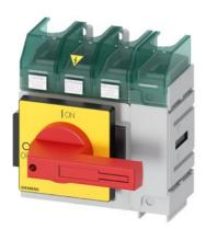
SENTRON, Molded case switch 3LD5 UL, Emergency switching-off, 4-pole, certified according to UL489 UL60947-4-1 and IEC60947-3, UL: 100A, SCCR 65kA at 480VAC, Operating power at 480VAC 3-phase: 60hp, IEC: 100A, Operating power at AC-23A at 400V: 45kW, floor mounting with direct handle, red/yellow, incl. terminal covers for the infeed side
