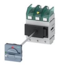
SENTRON, Molded case switch 3LD5 UL, Main switch, 3-pole, certified according to UL489 UL60947-4-1 and IEC60947-3, UL: 100A, SCCR 65kA at 480VAC, Operating power at 480VAC 3-phase: 60hp, IEC: 100A, Operating power at AC-23A at 400V: 45kW, floor mounting with door coupling rotary operating mechanism, defeatable, Standard, 4-hole mounting of the handle, without tolerance compensation, incl. terminal covers for the infeed side
