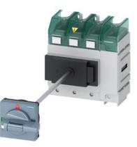
SENTRON, Molded case switch 3LD5 UL, Main switch, 4-pole, certified according to UL489 UL60947-4-1 and IEC60947-3, UL: 100A, SCCR 65kA at 480VAC, Operating power at 480VAC 3-phase: 60hp, IEC: 100A, Operating power at AC-23A at 400V: 45kW, floor mounting with door coupling rotary operating mechanism, defeatable, Standard, 4-hole mounting of the handle, without tolerance compensation, incl. terminal covers for the infeed side
