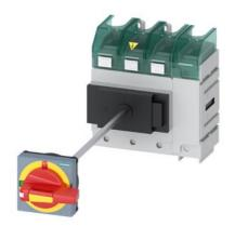
SENTRON, Molded case switch 3LD5 UL, Emergency switching-off, 4-pole, certified according to UL489 UL60947-4-1 and IEC60947-3, UL: 100A, SCCR 65kA at 480VAC, Operating power at 480VAC 3-phase: 60hp, IEC: 100A, Operating power at AC-23A at 400V: 45kW, floor mounting with door coupling rotary operating mechanism, defeatable, emergency switching-off, 4-hole mounting of the handle, without tolerance compensation, incl. terminal covers for the infeed side
