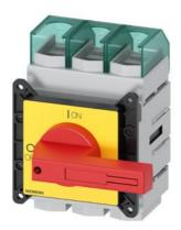
SENTRON, Molded case switch 3LD5 UL, Emergency switching-off, 3-pole, certified according to UL489 UL60947-4-1 and IEC60947-3, UL: 100A, SCCR 65kA at 480VAC, Operating power at 480VAC 3-phase: 60hp, IEC: 100A, Operating power at AC-23A at 400V: 45kW, front-mounted, rotary operating mechanism, red/yellow, 4-hole mounting of the handle, incl. terminal covers for the infeed side
