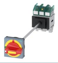
SENTRON, Molded case switch 3LD5 UL, Emergency switching-off, 3-pole, certified according to UL489 UL60947-4-1 and IEC60947-3, UL: 60A, SCCR 50kA at 480VAC, Operating power at 480VAC 3-phase: 40hp, IEC: 63A, Operating power at AC-23A at 400V: 30kW, floor mounting with door coupling rotary operating mechanism, defeatable, emergency switching-off, 4-hole mounting of the handle, without tolerance compensation, incl. terminal covers for the infeed side
