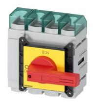
SENTRON, Molded case switch 3LD5 UL, Emergency switching-off, 4-pole, certified according to UL489 UL60947-4-1 and IEC60947-3, UL: 100A, SCCR 65kA at 480VAC, Operating power at 480VAC 3-phase: 60hp, IEC: 100A, Operating power at AC-23A at 400V: 45kW, front-mounted, rotary operating mechanism, red/yellow, 4-hole mounting of the handle, incl. terminal covers for the infeed side
