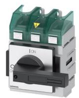
SENTRON, Molded case switch 3LD5 UL, Main switch, 3-pole, certified according to UL489 UL60947-4-1 and IEC60947-3, UL: 125A, SCCR 65kA at 480VAC, Operating power at 480VAC 3-phase: 75hp, IEC: 125A, Operating power at AC-23A at 400V: 55kW, floor mounting with direct handle, black, incl. terminal covers for the infeed side
