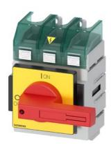
SENTRON, Molded case switch 3LD5 UL, Emergency switching-off, 3-pole, certified according to UL489 UL60947-4-1 and IEC60947-3, UL: 125A, SCCR 65kA at 480VAC, Operating power at 480VAC 3-phase: 75hp, IEC: 125A, Operating power at AC-23A at 400V: 55kW, floor mounting with direct handle, red/yellow, incl. terminal covers for the infeed side
