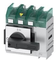
SENTRON, Molded case switch 3LD5 UL, Main switch, 4-pole, certified according to UL489 UL60947-4-1 and IEC60947-3, UL: 125A, SCCR 65kA at 480VAC, Operating power at 480VAC 3-phase: 75hp, IEC: 125A, Operating power at AC-23A at 400V: 55kW, floor mounting with direct handle, black, incl. terminal covers for the infeed side
