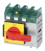
SENTRON, Molded case switch 3LD5 UL, Emergency switching-off, 4-pole, certified according to UL489 UL60947-4-1 and IEC60947-3, UL: 125A, SCCR 65kA at 480VAC, Operating power at 480VAC 3-phase: 75hp, IEC: 125A, Operating power at AC-23A at 400V: 55kW, floor mounting with direct handle, red/yellow, incl. terminal covers for the infeed side
