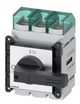
SENTRON, Molded case switch 3LD5 UL, Main switch, 3-pole, certified according to UL489 UL60947-4-1 and IEC60947-3, UL: 125A, SCCR 65kA at 480VAC, Operating power at 480VAC 3-phase: 75hp, IEC: 125A, Operating power at AC-23A at 400V: 55kW, front-mounted, rotary operating mechanism, black, 4-hole mounting of the handle, incl. terminal covers for the infeed side
