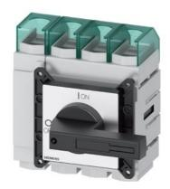
SENTRON, Molded case switch 3LD5 UL, Main switch, 4-pole, certified according to UL489 UL60947-4-1 and IEC60947-3, UL: 125A, SCCR 65kA at 480VAC, Operating power at 480VAC 3-phase: 75hp, IEC: 125A, Operating power at AC-23A at 400V: 55kW, front-mounted, rotary operating mechanism, black, 4-hole mounting of the handle, incl. terminal covers for the infeed side
