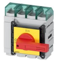
SENTRON, Molded case switch 3LD5 UL, Emergency switching-off, 4-pole, certified according to UL489 UL60947-4-1 and IEC60947-3, UL: 125A, SCCR 65kA at 480VAC, Operating power at 480VAC 3-phase: 75hp, IEC: 125A, Operating power at AC-23A at 400V: 55kW, front-mounted, rotary operating mechanism, red/yellow, 4-hole mounting of the handle, incl. terminal covers for the infeed side
