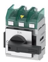
SENTRON, Molded case switch 3LD5 UL, Main switch, 3-pole, certified according to UL489 UL60947-4-1 and IEC60947-3, UL: 150A, SCCR 50kA at 480VAC, Operating power at 480VAC 3-phase: 100hp, IEC: 160A, Operating power at AC-23A at 400V: 75kW, floor mounting with direct handle, black, incl. terminal covers for the infeed side
