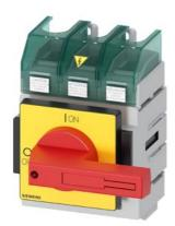
SENTRON, Molded case switch 3LD5 UL, Emergency switching-off, 3-pole, certified according to UL489 UL60947-4-1 and IEC60947-3, UL: 150A, SCCR 50kA at 480VAC, Operating power at 480VAC 3-phase: 100hp, IEC: 160A, Operating power at AC-23A at 400V: 75kW, floor mounting with direct handle, red/yellow, incl. terminal covers for the infeed side
