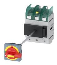
SENTRON, Molded case switch 3LD5 UL, Emergency switching-off, 3-pole, certified according to UL489 UL60947-4-1 and IEC60947-3, UL: 150A, SCCR 50kA at 480VAC, Operating power at 480VAC 3-phase: 100hp, IEC: 160A, Operating power at AC-23A at 400V: 75kW, floor mounting with door coupling rotary operating mechanism, defeatable, emergency switching-off, 4-hole mounting of the handle, without tolerance compensation, incl. terminal covers for the infeed side
