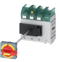
SENTRON, Molded case switch 3LD5 UL, Emergency switching-off, 4-pole, certified according to UL489 UL60947-4-1 and IEC60947-3, UL: 150A, SCCR 50kA at 480VAC, Operating power at 480VAC 3-phase: 100hp, IEC: 160A, Operating power at AC-23A at 400V: 75kW, floor mounting with door coupling rotary operating mechanism, defeatable, emergency switching-off, 4-hole mounting of the handle, without tolerance compensation, incl. terminal covers for the infeed side
