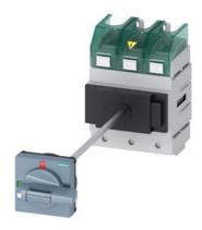
SENTRON, Molded case switch 3LD5 UL, Main switch, 3-pole, certified according to UL489 UL60947-4-1 and IEC60947-3, UL: 150A, SCCR 50kA at 480VAC, Operating power at 480VAC 3-phase: 100hp, IEC: 160A, Operating power at AC-23A at 400V: 75kW, floor mounting with door coupling rotary operating mechanism, defeatable, Standard, 4-hole mounting of the handle, without tolerance compensation, incl. terminal covers for the infeed side
