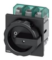
SENTRON, Molded case switch 3LD5 UL, Main switch, 3-pole, certified according to UL489 UL60947-4-1 and IEC60947-3, UL: 60A, SCCR 50kA at 480VAC, Operating power at 480VAC 3-phase: 40hp, IEC: 63A, Operating power at AC-23A at 400V: 30kW, front-mounted, rotary operating mechanism, black, 4-hole mounting of the handle, incl. terminal covers for the infeed side
