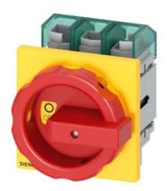
SENTRON, Molded case switch 3LD5 UL, Emergency switching-off, 3-pole, certified according to UL489 UL60947-4-1 and IEC60947-3, UL: 60A, SCCR 50kA at 480VAC, Operating power at 480VAC 3-phase: 40hp, IEC: 63A, Operating power at AC-23A at 400V: 30kW, front-mounted, rotary operating mechanism, red/yellow, 4-hole mounting of the handle, incl. terminal covers for the infeed side
