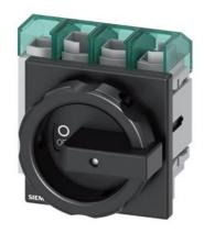
SENTRON, Molded case switch 3LD5 UL, Main switch, 4-pole, certified according to UL489 UL60947-4-1 and IEC60947-3, UL: 60A, SCCR 50kA at 480VAC, Operating power at 480VAC 3-phase: 40hp, IEC: 63A, Operating power at AC-23A at 400V: 30kW, front-mounted, rotary operating mechanism, black, 4-hole mounting of the handle, incl. terminal covers for the infeed side
