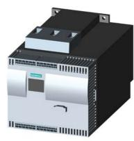
SIRIUS soft starter Values at 400 V, 40 °C standard: 47 A, 22 kW Inside-delta: 81 A, 45 kW 200-460 V AC, 230 V AC spring-type terminals !!! Phased-out product !!! Successor is SIRIUS 3RW5, Preferred successor type is >>3RW5524-3HA14<<
